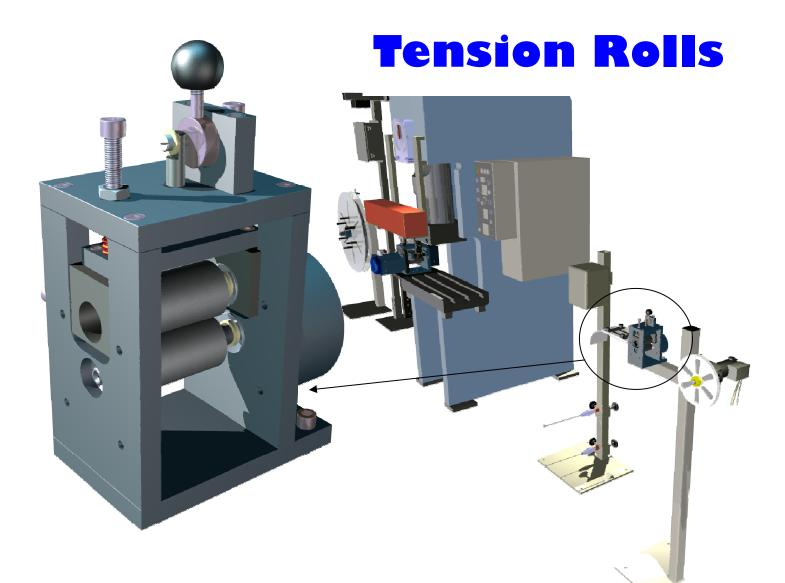
Small tension roll assembly for tightly rewound coils
