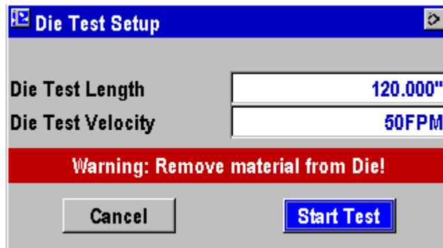
Figure 6-22. Die Test Popup with Warning
